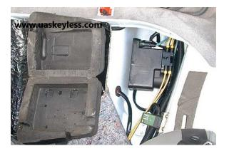
Pry up on the retaining clip that holds the vacuum supply lines to free vacuum line connector from the pump. This will give you easier access to the pump since there is truly little slack in the vacuum lines. Be incredibly careful not to break this clip.
