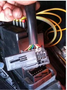
Use a utility knife and carefully cut the black sleeve on the wiring harness to expose the wires.
