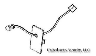
NOTE: Should the LED fit loosely into the drilled hole, it can be secured in place with a carefully applied drop of "super glue" (not supplied in kit) applied on the backside of the knockout panel.
