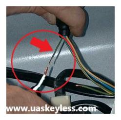
© Copyright 2021-2025 United Auto Security, LLC. All Rights Reserved. Unauthorized reproduction, or distribution of this manual, or any portion of it is strictly prohibited. Connect the White/Black wire from the keyless harness to the Green wire side away from the vacuum pump, using the supplied Heat Shrink with Solder connector.
