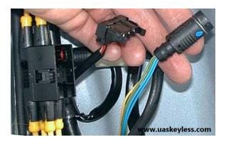
Find the 2 green wires on the round connector. It depends on the pump your Benz has, you might have a duplicate wire colors, that is why the next step is important. Pick one of the green wires and check to see if it is the correct wire using the voltmeter.
