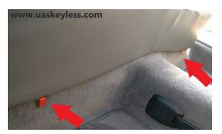
Remove the carpeting on the right (passenger's) side to gain access to the door locking vacuum pump. The pump is encased in a foam mold. Remove the pump from the foam mold by sliding the foam enclosure rearwards until it is free. Open the enclosure and slide away from the pump.
