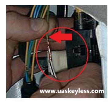
Black Wire: Connect this wire to Ground (Vehicle Frame Directly using the supplied self-tapping screw) or Brown wire @ the Rectangular plug.
