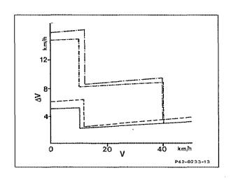
Slip thresholds (When both drive wheels skid)
