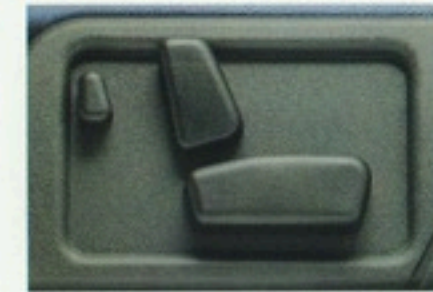
The ingenious Mercedes seat-adjustment switch, shaped like the seat itself, allows for precise control with minimal effort.
