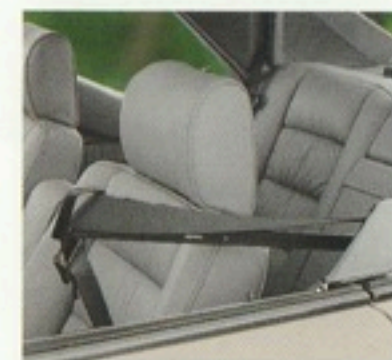
Front seat belts are offered to driver and front-seat passenger by means of automatic electric presenters which retract once the belts are fastened.
