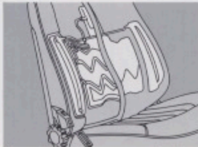
Seats with electro-pneumatically adjusted orthopedic backrests.
