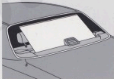
A rear window sunshade helps prevent excessive cabin heat.
