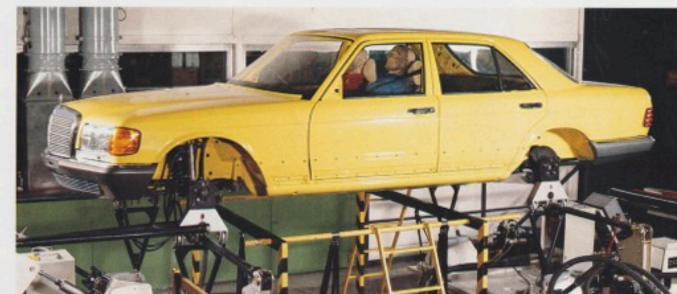
This hydraulically operated rig is an important tool in the quest for more durable and reliable cars. When activated, it mercilessly shakes developmental prototypes in order to pinpoint components or fasteners that might possibly rattle loose or fail by fatigue.
