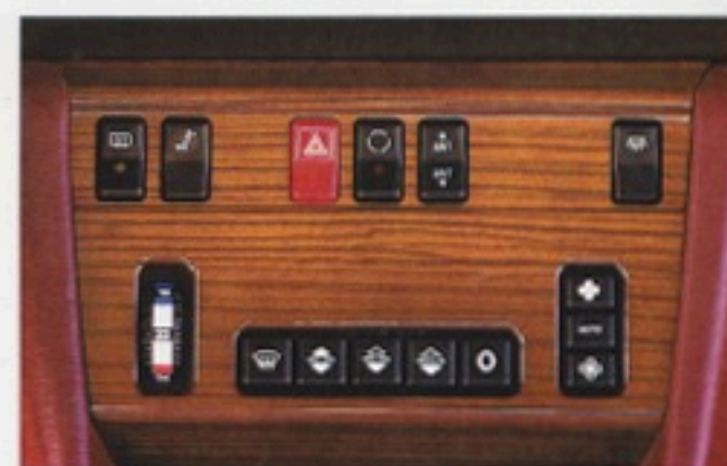
Interior temperature, air distribution and air volume are controlled as part of the fully automatic climate control system. Ventilation outlets for right and left front sides of the interior can be individually set. Cabin air is exchanged approximately three times per minute with the blower set at high speed. Set the system once to the temperature level you prefer and it can maintain it continuously, year-round.
