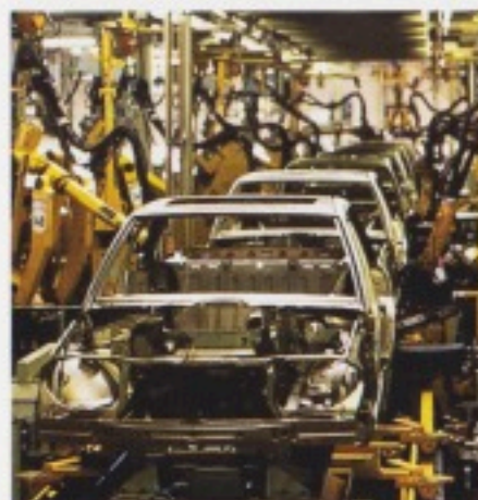
While hand workmanship remains intensive, Mercedes-Benz also relies on the inhumanly tireless and precise resource of advanced robotics in the assembly process, as with the robot welders above.
