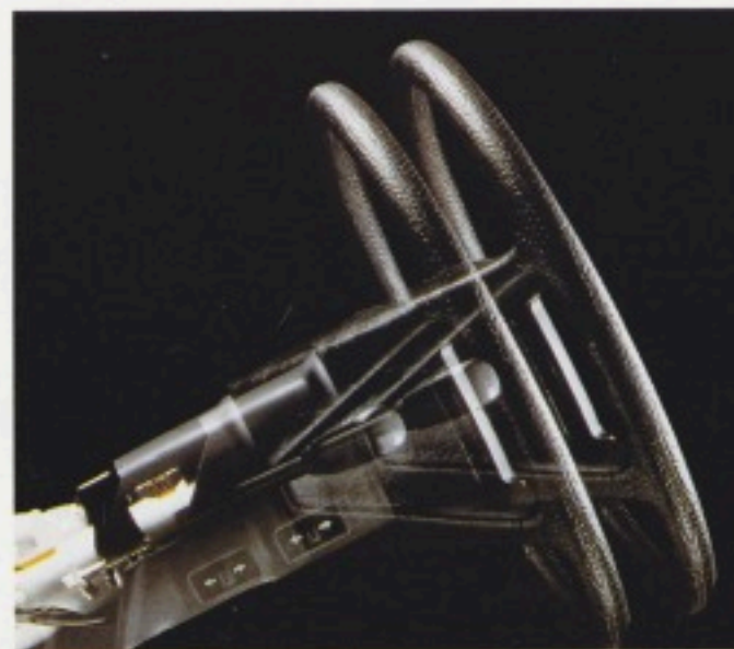
The steering wheel in the 300E, 300D Turbo and 300TD Turbo is electrically adjustable through a total of 2.36 inches of fore and aft travel. The column-mounted controls move with it.
