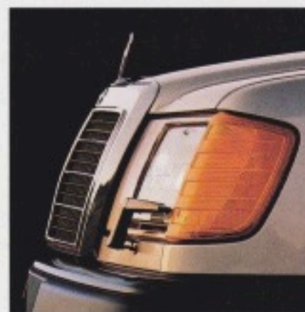
European-style headlamp wipers and washers are fitted to the 300E as standard equipment.
