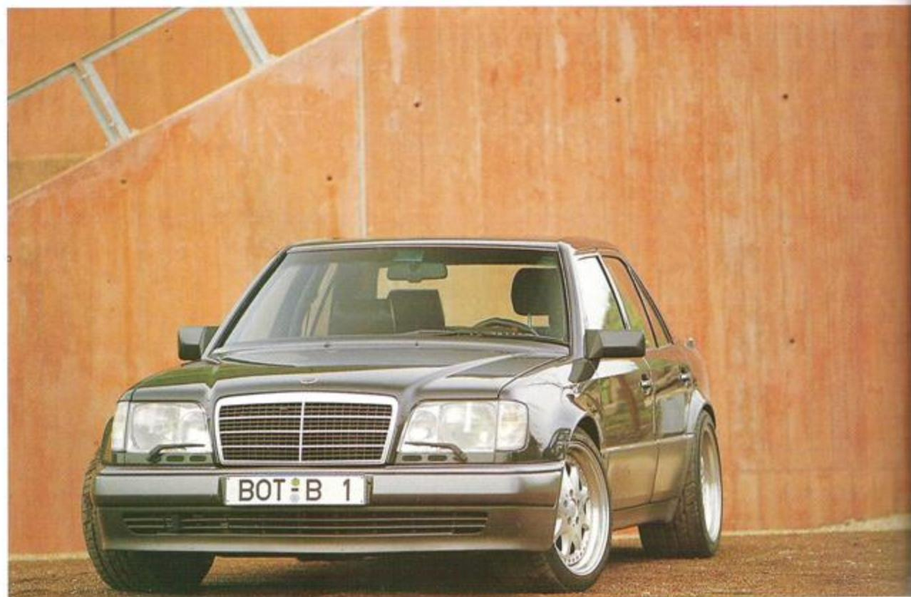
Transplanting their 7.3-48 engine into the Mercedes-Benz W124 E500, a car already acknowledged as a paragon of understated performance, BRABUS have produced the fastest four-door saloon in the world. With the power and torque of the consummate Mercedes-Benz sports saloon raised to 530 bhp at 5700 rpm and 755 Nm (557 ft lb) of torque at 3700rpm, it is a veritable sledgehammer, Arnold Schwarzenegger in an Armani suit!
