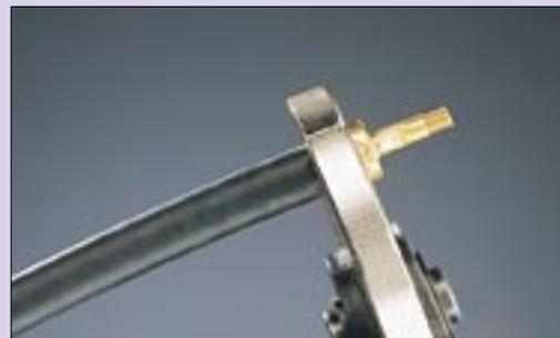
**4** The connection between the sleeve and silicon outer sleeve is created during the second crimping process. Use the crimping pliers in position 1. Insert the sleeve in such a way that it closes together with the rear edge of the pliers, then press the pliers together until they self-release.
