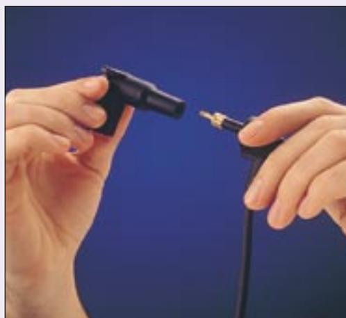
**6** Finally, screw on the ignition distributor connector of the CopperCable.
