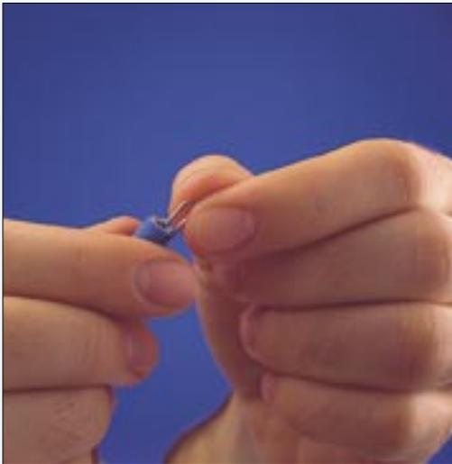
2 Insert the contact pin into the cable between the insulation and resistor wire.
