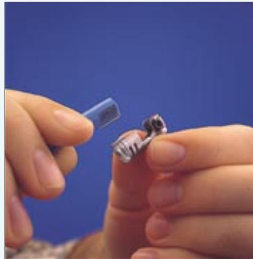
3 Insert sleeve into the cable (contact pin on the sleeve).
