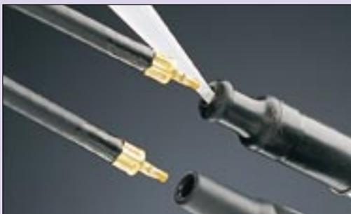
**5** Fitting the spark plug connector or the ignition distribution connector: apply installation oil to the ignition cable and the internal silicon seal on the connector.
