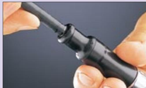
**6** The ignition cable must now be screwed into the connector. Finally, unscrew it by one quarter revolution to make it easier to subsequently unscrew the connector.
