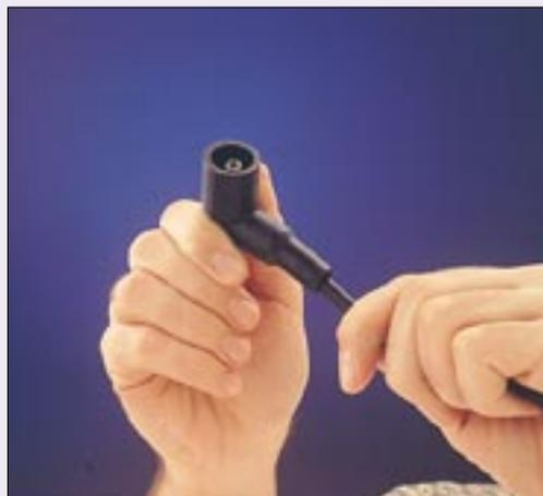
**2** Unscrew the ignition distributor plug on the new CopperCable (spray with Beru installation oil).
