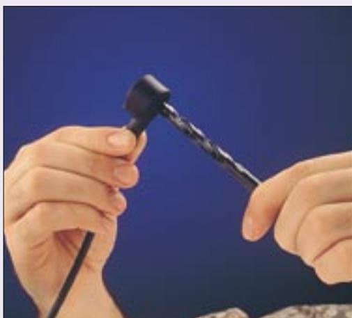
**3** Drill 8 mm hole on the pulse timer (turn drill by hand).
