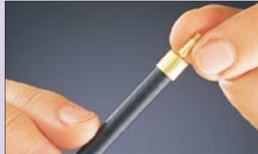
**2** Now carefully position the M3 threaded sleeve onto the ignition cable. We recommend that you twist the fine copper wires slightly beforehand so they do not splay out when being connected, instead they all slot into the threaded section of the connection sleeve.
