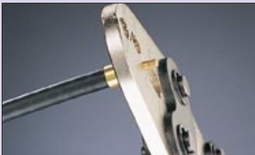
**3** To produce the connection between sleeve and copper core, proceed as follows: first place the ignition cable with sleeve into the crimping pliers - so that the thread protrudes out of the plier jaws. Then press the pliers together until they self-release.
