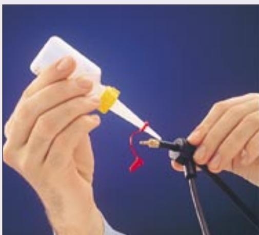
**5** Now lubricate the ignition cable with installation oil.
