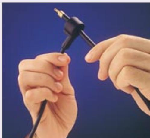
**4** The ignition cable with the M3 connection can now be pushed through the pulse timer.
