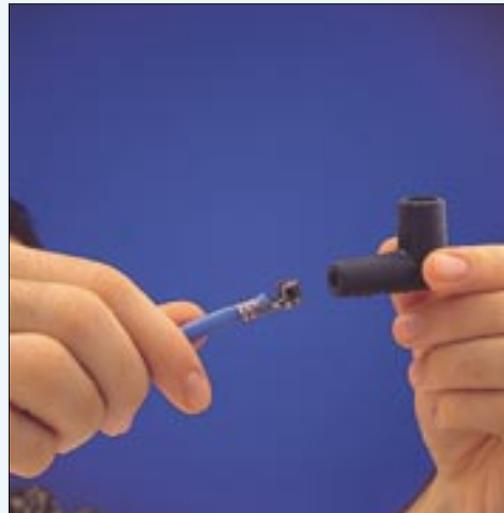
5 then, with the help of the tool and installation oil, slide into the waterproof cover on the spark plug connector from below.
