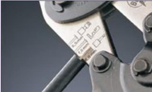
**1** Remove the insulation at the end of the ignition cable with the help of an appropriate tool (wire cutter). An easy way to check the correct length of cable has been stripped, i.e. 6.8 mm, is to place it in the head of the pliers.
