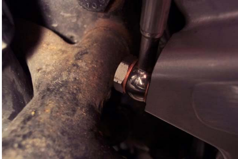
The next thing i modified was the heat shields. I used the ones that are fitted to SL 129 with the 334mm discs.
