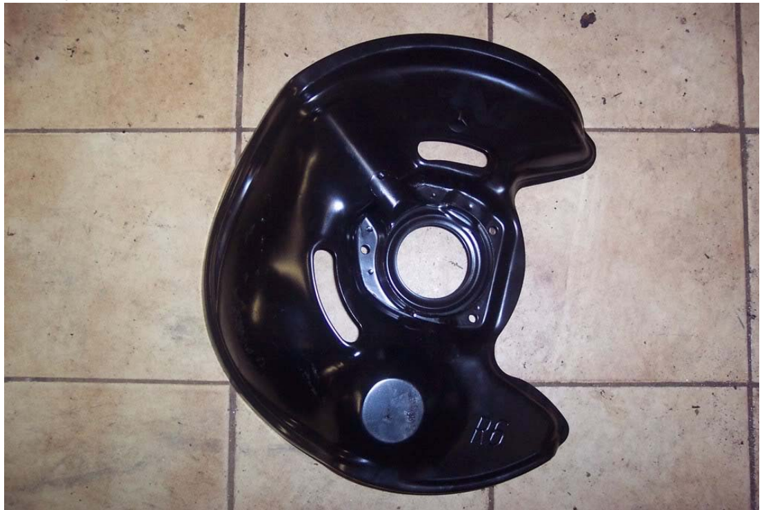
You have to cut them were the caliper fits. Then repaint the edges.
