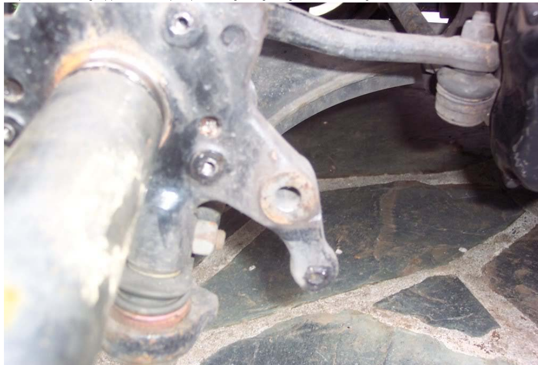
This has to be cut of and rounded of around caliper lower bolt hole.
