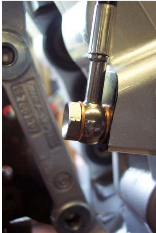
Heres a close up banjo connection and position of steering arm.
