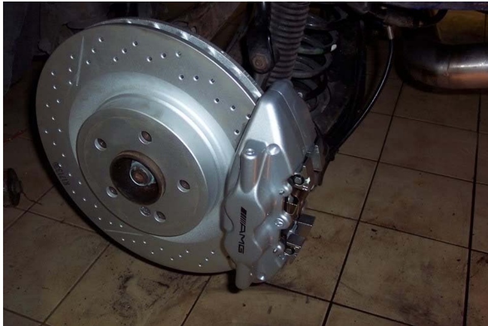
The caliper and disc fit perfectly with no spacers. bolt straight on. Heres the finished job with braided brake lines.
