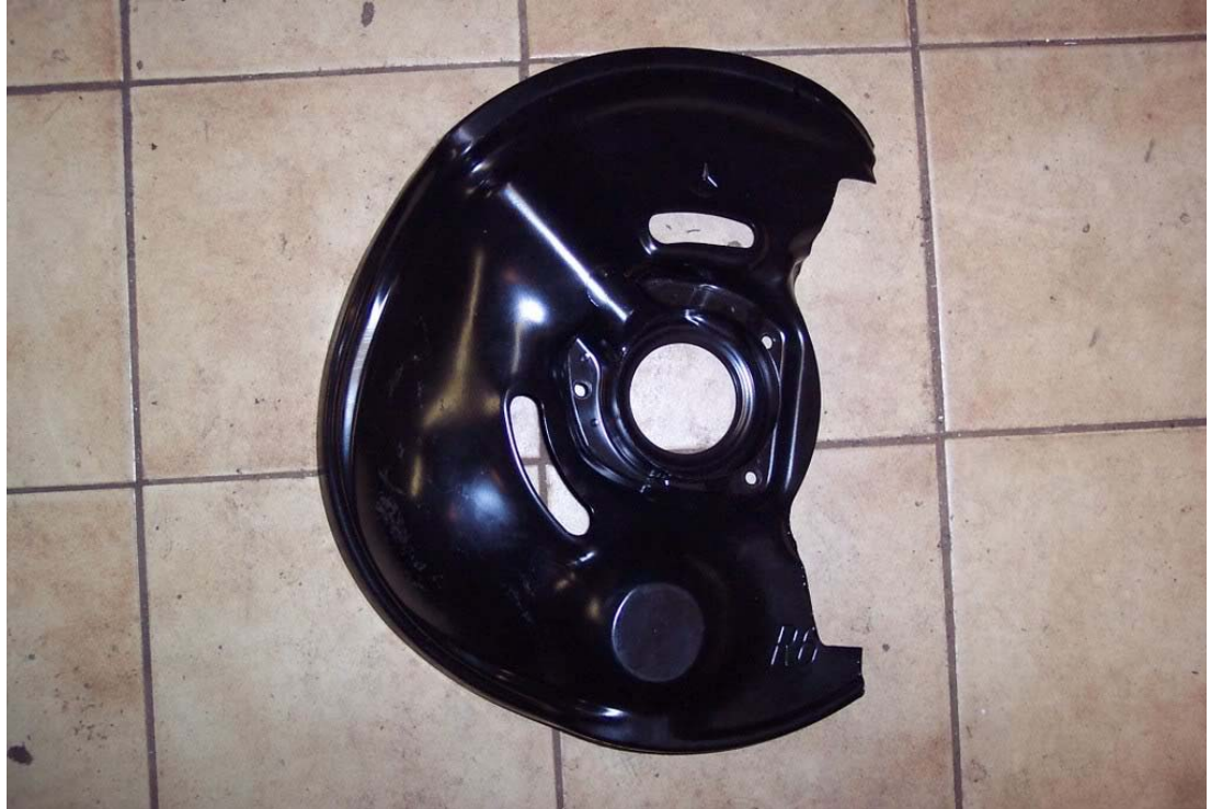
So now we can assemble, on with heat shield, back on with hub.
