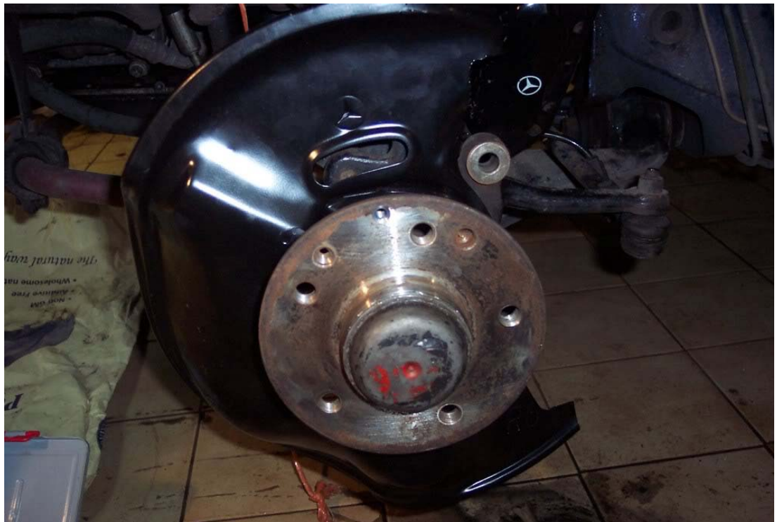
Now on with disc, forgot the maintenance bolt that holds disc to the hub is in a different place. I have redrilled the hub as can be seen in the last photo. Decided better instead of disc every time you change discs.
