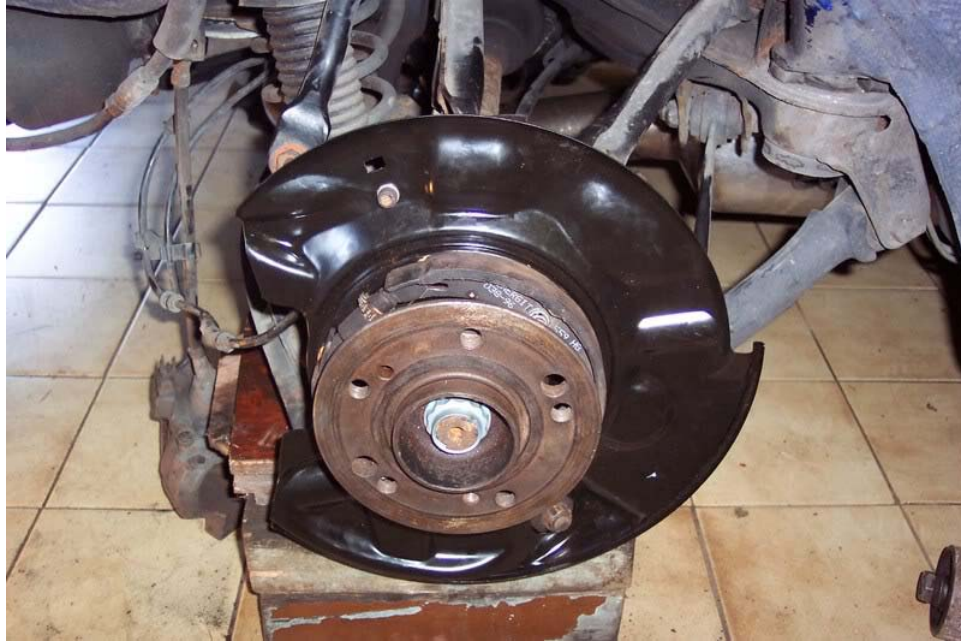
The caliper and disc fit perfectly with no spacers. bolt straight on. Heres the finished job with braided brake lines.
